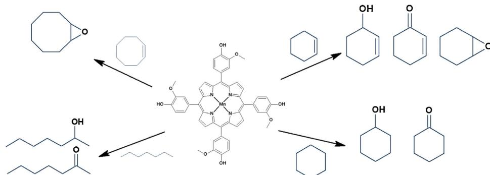
**Fig. 4.** Schematic representation of the oxidation of hydrocarbons catalyzed by the MnP studied herein (clockwise): *cis*-cyclooctene, cyclohexene, cyclohexane, and *n*-heptane.
