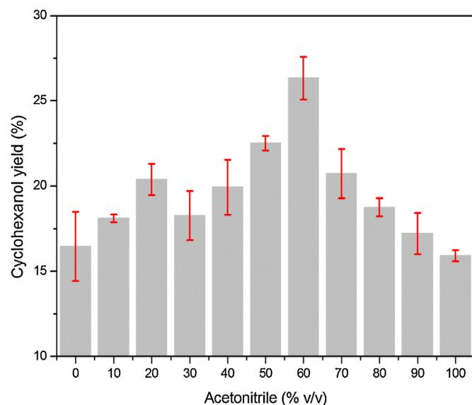
Fig. 5. Dependence of the cyclohexanol yield on the composition of the solvent mixture.
