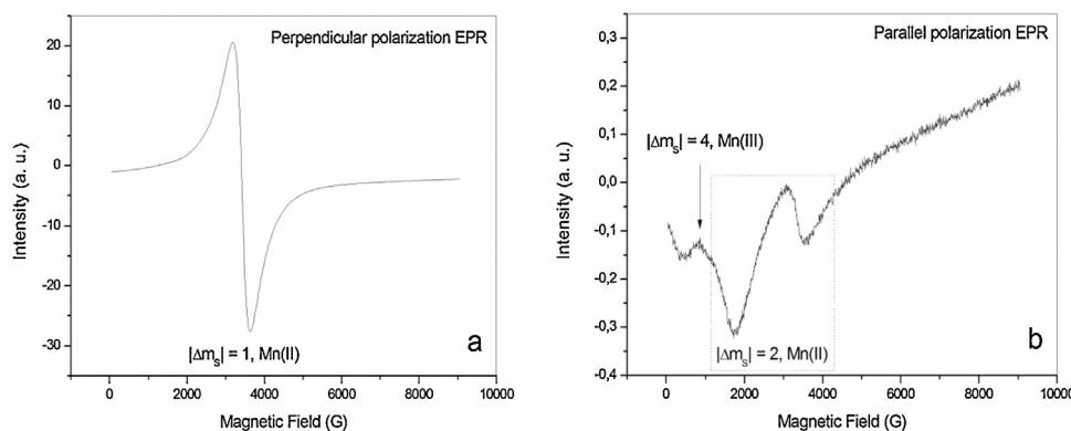
**Fig. 2.** 77-K X-band EPR MnPS spectra. (a) Perpendicular polarization. The intense absorption around 3500 G, characteristic of Mn(II) species, is due to a  $\Delta m_s = \pm 1$  selection rule transition. (b) Parallel polarization. The  $\Delta m_s = \pm 4$  transition, present as an absorption around 900 G, is due to Mn(III) species. The Mn(II) species also produce  $\Delta m_s = \pm 2$  absorptions in the parallel polarization EPR experiment (B, dashed rectangle).
