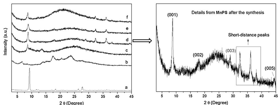
**Fig. 3.** Powder X-ray diffraction patterns of (a)  $\text{Mn}(\text{OAc})_2$ , (b) HP, (c) MnP, (d) MnPS after synthesis, (e) MnPS after de-solvation under vacuum, and (f) MnPS after re-solvation with DMF.
